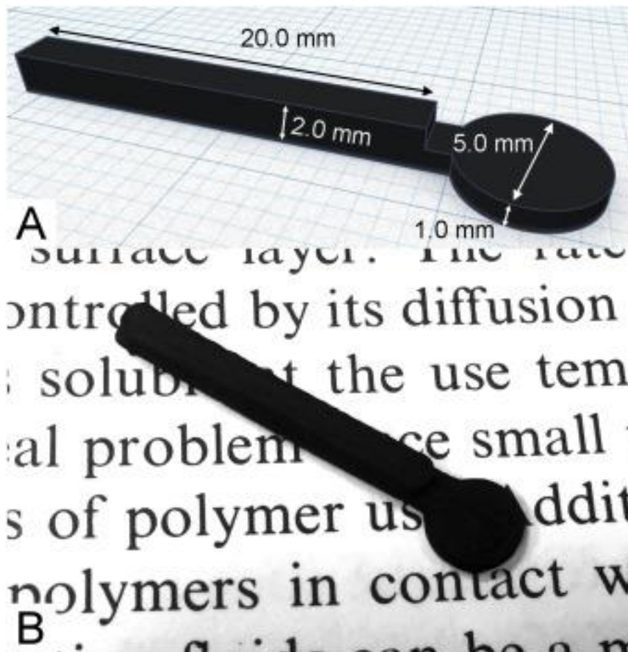
Figure 5. (a) The design drawn in the Tinkercad platform and (b) the digital photo of the 3D graphene electrode. (Reprinted from [23] with permission of Elsevier).
